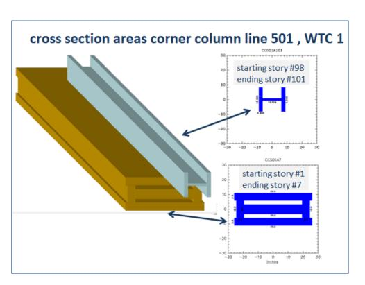
corner columns that were located between the 12<sup>th</sup> and the 41<sup>st</sup> stories.<sup>87</sup> The cross-section-length-to-plate-thickness ratio of this column corresponds most closely to core corner columns that spanned stories 24 to 30.<sup>88</sup> The column is one of the many documented pieces of structural steel<sup>89</sup> that contradict Khalezov's "dustification" claim.
