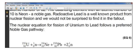
The mass ratio of the two daughter nuclei in this reaction, allegedly occurring in nuclear blasts, is 1 to 8.75 (instead of about 2 to 3). Even the diagram Tahil uses (see screen shot in footnote 46) shows that lead, which has 82 protons, is too heavy to be a product of neutron-induced fission (see also footnote 43). Lead is the end product of natural decay chains; these natural processes do not produce nuclear blasts.
