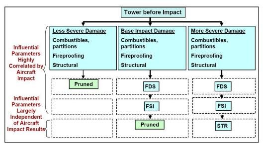
Figure 9-3. Pruned analysis tree for influential parameter effects.
