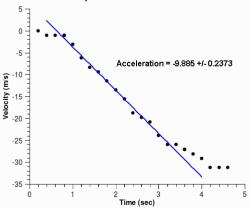
Velocity vs Time for NW Corner of WTC7
