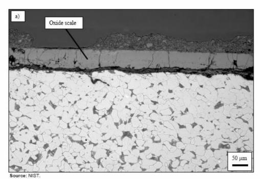
Figure 6–12. Light optical micrographs of the microstructure of a perimeter floor truss seat from the 99th floor of WTC 1, panel N-8 (A142: 97-100). a) Ferrite-pearlite microstructure and developed oxide scale. Two percent nital and 4 percent picral etch.
