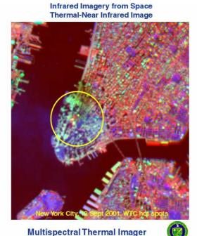
The thermal-near infrared image is a combination of thermal infrared (red), short-wave infrared (green) and near-infrared (blue). This image has approximately 20-meter resolution. The smoke is more transparent in the infrared bands than for a visible image. This image shows differences between the four hotspots in the disaster area due to temperature variations. The hottest areas are yellow and a slightly cooler hotspot is red-orange.
