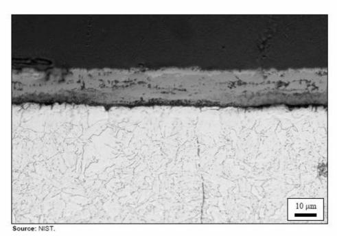
Figure 6–8. Iron oxide scale that developed on a 100 ksi quenched-and-tempered flange plate after isothermal exposure at 625 °C for 2 h. Sample was from panel C-10 (WTC 1, column 451, 88th floor). Two percent nital and 4 percent picral etch.
