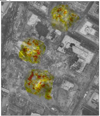
Note: Thermal data are overlaid on an orthophotograph obtained on October 8th. Variations in temperature are evident across the site. However, these values were acquired (and are therefore displayed) using an 8-bit radiometric scale, rather than an absolute calibration such as degrees Fahrenheit
