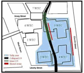
The New York City Department of Design and Construction (DDC) has divided the site into four quadrants for recovery operations and debris removal. Tully Construction, a heavy construction contractor experienced in emergency contracts, has the largest quadrant, encompassing nearly half the site. Included in Tully's zone are the South Tower and World Trade Center Buildings Four and Five.
