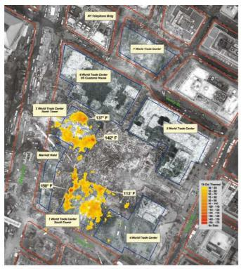
Fig. 5 Thermal data collected over the World Trade Center site on October 18, 2001, overlaid on digital orthophotography collected on October 7, 2001. Building footprints are shown in blue and streets are shown in 2001.
