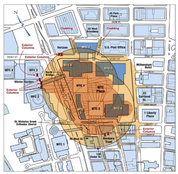
Figure 1-7 Schematic depiction of areas of collapse debris impact, based on aerial photographs and documented damage.
