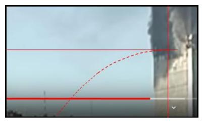
Figure 19: Starting location of the perimeter column wall section at the 80<sup>th</sup> floor of the east face as imputed from the horizontal and vertical velocities and accelerations.
