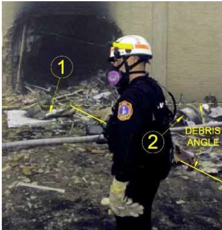
Figure AppE-4 Plane parts and debris angle
