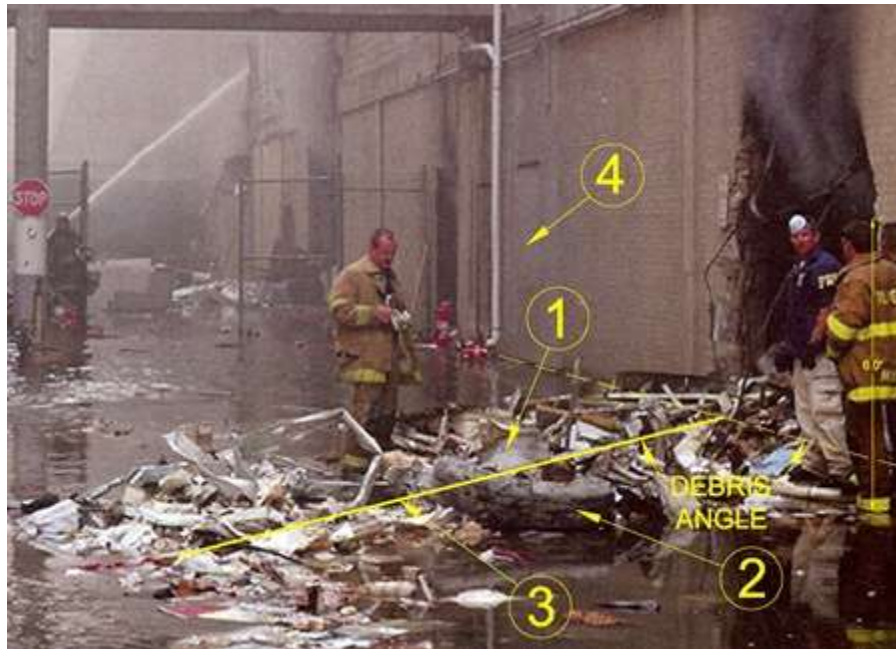
Figure AppE-5 Plane parts and debris angle
